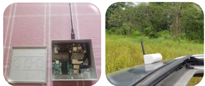
Fig. 2. Gateway Prototype and Data Collection IoT Node
